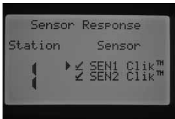
Both sensors programmed for Station 1
