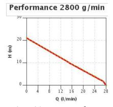
Characteristics referring to operation with water at 20  $^{\circ}$
