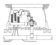
Plastic Electric Remote Control PGA Valve (with PRS-D) using side inlet
