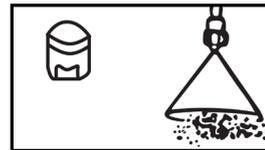
**Conical spray head:** Suitable for spraying pesticide and insecticide.
